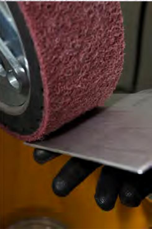
Norton Rapid Prep surface conditioning belts provide better performance and longer life versus conventional surface conditioning belts. These belts are ideal for removing surface defects, edge burrs, parting lines or flashing, rust, oxides, corrosion, paints and scale, cleaning molds, blending mill marks, tool marks, uneven edges and refining coated abrasive finish.
